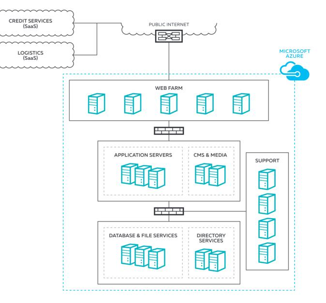
As shown in the diagram, not much has changed in the environment's overall design. In actual implementation, the firewalls are replaced by Azure network security groups (NSGs) within the virtual network. But this is a one-for-one, server-to-VM scenario that minimizes
